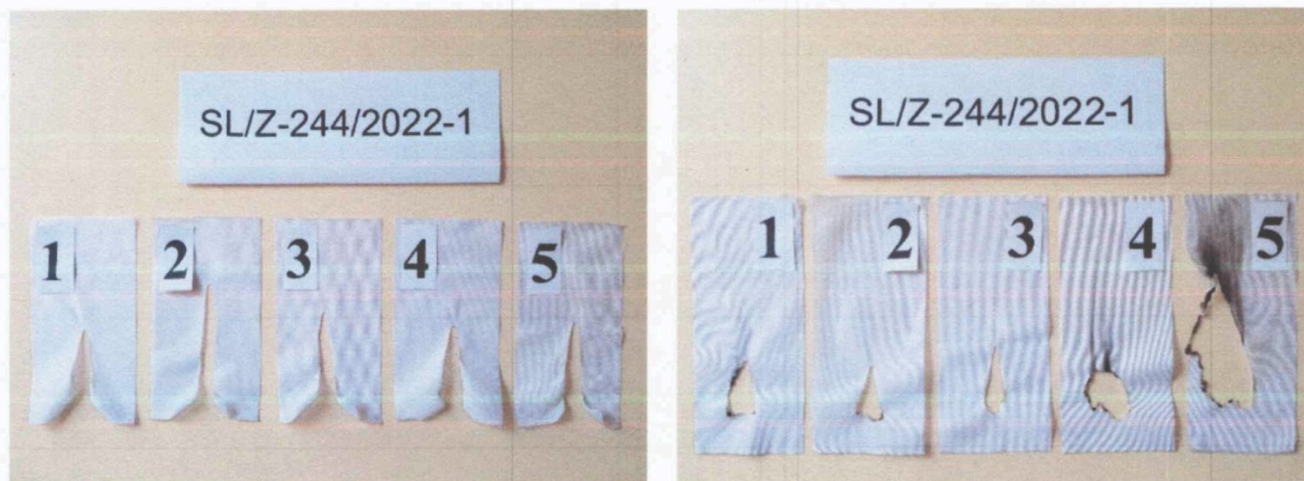
Figure 5. Appearance of the sample after the small burner test - ART: 101704/BC/WPL/OG (length direction)
